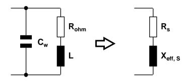
ohm's resistance of the antenna  $[\Omega]$
